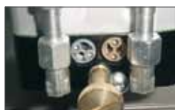
By pass valves for the force adjustment
