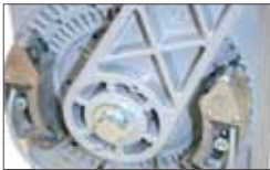
Adjustable mechanical and electronic limit switches in opening and closing (only for FLIPPER PLUS)
