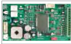
USER 1 - 24V DG control unit programmable with Led display and integrated warning light.
